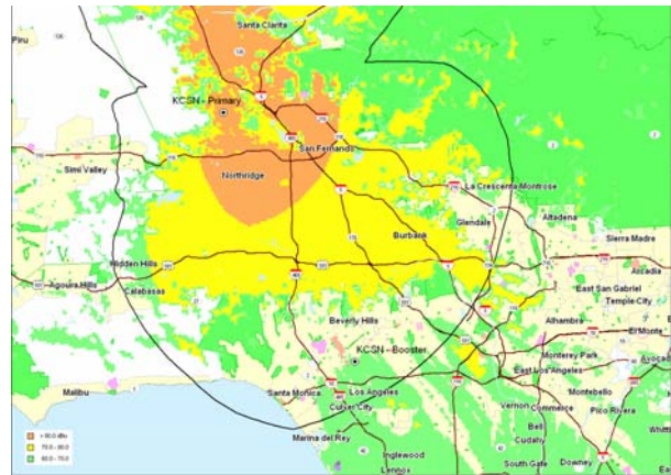
Figure 9 KCSN(FM) primary analog coverage area (part); green is 60-70 dBu. This Longley-Rice coverage prediction shows a sharp cutoff of coverage to the south. Central Los Angeles is in the lower right of the map.
